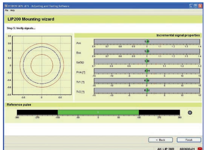
Commissioning via the PWM 21 and ATS software
