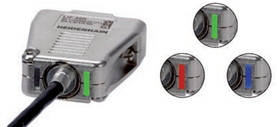
LIF, LIP 6071: function indicator in the interface electronics
