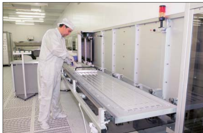
Vacuum machine for application of chromium layers
