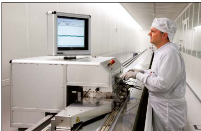
30 m long measuring machine for scale tapes
