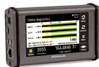
PWT 100 test device for mobile application
