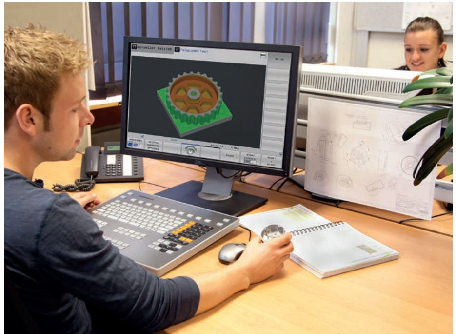
Programming station with TNC operating panel
