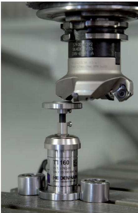
Measuring the tool length
