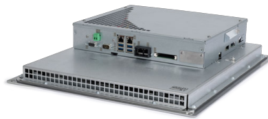
MC 8512 with main computer installed on the back
